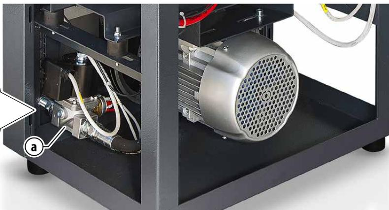
**WARNING:** The shut-off solenoid valve (a) must be replaced every 5 years or 3000 hours.
