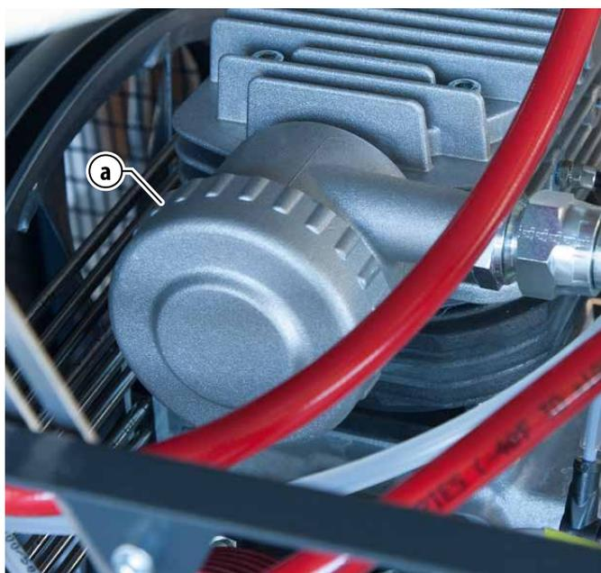
**7.6 SOSTITUZIONE FILTRO DI ASPIRAZIONE**
